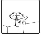
7. Insert speaker into mounting hole. Tighten both screws on the baffle face to actuate the mounting wings. DO NOT OVERTIGHTEN.
